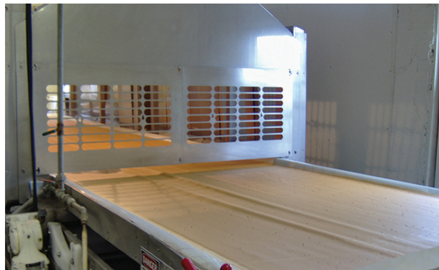
The Refractance Window dryer uses simple principles of convection, conduction and infrared energy from hot water instead of high heat.
